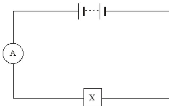
As component **X** is heated, the reading on the ammeter goes up.
