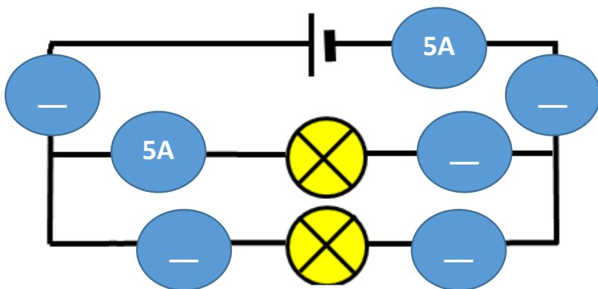
Label the diagram with the current at each point
