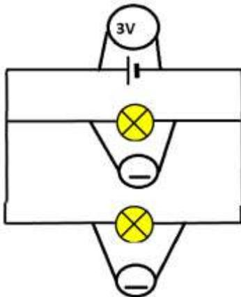
Label the diagram with the voltage at each point
